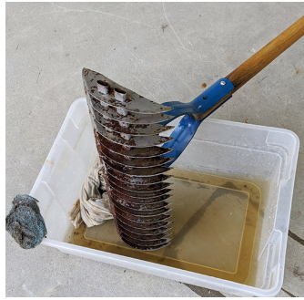
Removing rust with vinegar
