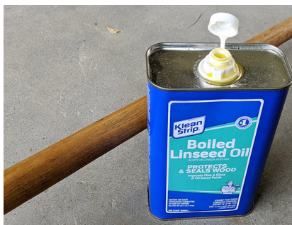
Coat wooden handle with linseed oil
